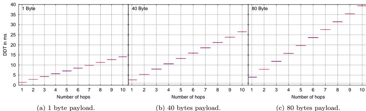
Figure 1: Deterministic Delivery Time (DDT) for different payload sizes.
